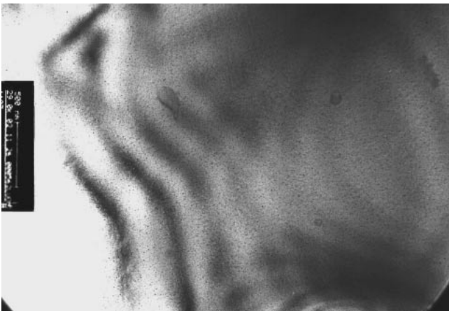
Fig. 3. Plan-view TEM image of the top Ge layer.
