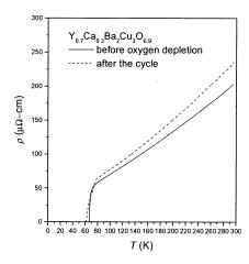
Fig. 1.  $\rho(T)$  of the Ca-doped YBCO shows a nearly complete recovery from the oxygen depletion.
