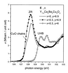
Fig. 2. O K-edge XANES for  $\mathbf{E} \perp c$ . While Ca doping leads to an increase in the ZR band spectral weight associated with the CuO2 planes in  $Y_{0.7}Ca_{0.3}Ba_2Cu_3O_{6.9}$ , this doping effect is absent in  $Y_{0.7}Ca_{0.3}Ba_2Cu_3O_{6.9}$ .
