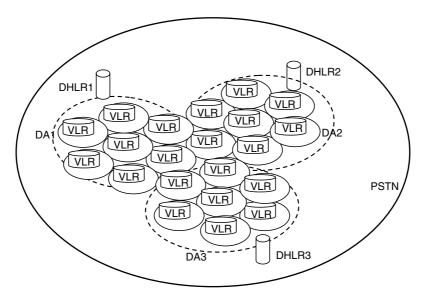
Fig. 1. Distributed HLRs architecture.
