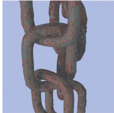
Fig. 11. Rust on ferrous chains
