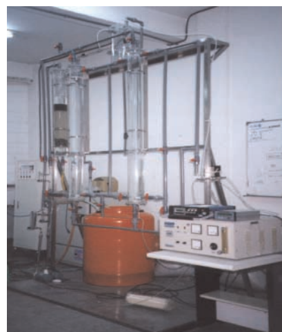
Figure 2. The apparatus of sand filter and ozonation setup.
