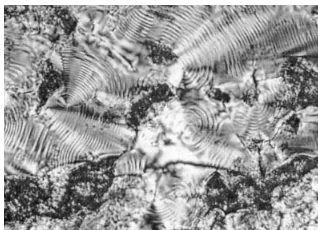
Figure 1. Optical polarizing micrograph of PS112Bs15 revealing SmC* phase at 96^\circ\text{C} (800 \times ).
