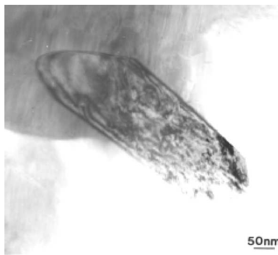
Fig. 10. TEM bright field (BF) image of system A annealed at 700°C for 2 h.
