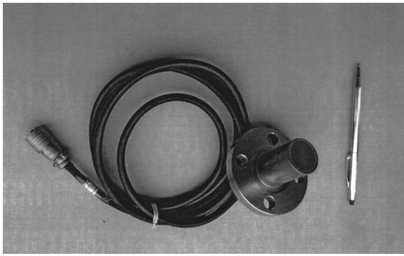
Fig. 5. Soil pressure transducer
