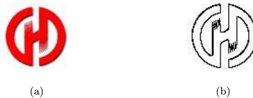
Fig. 8. The result of edge detection. (a) A color trademark. (b) Edges detected.
