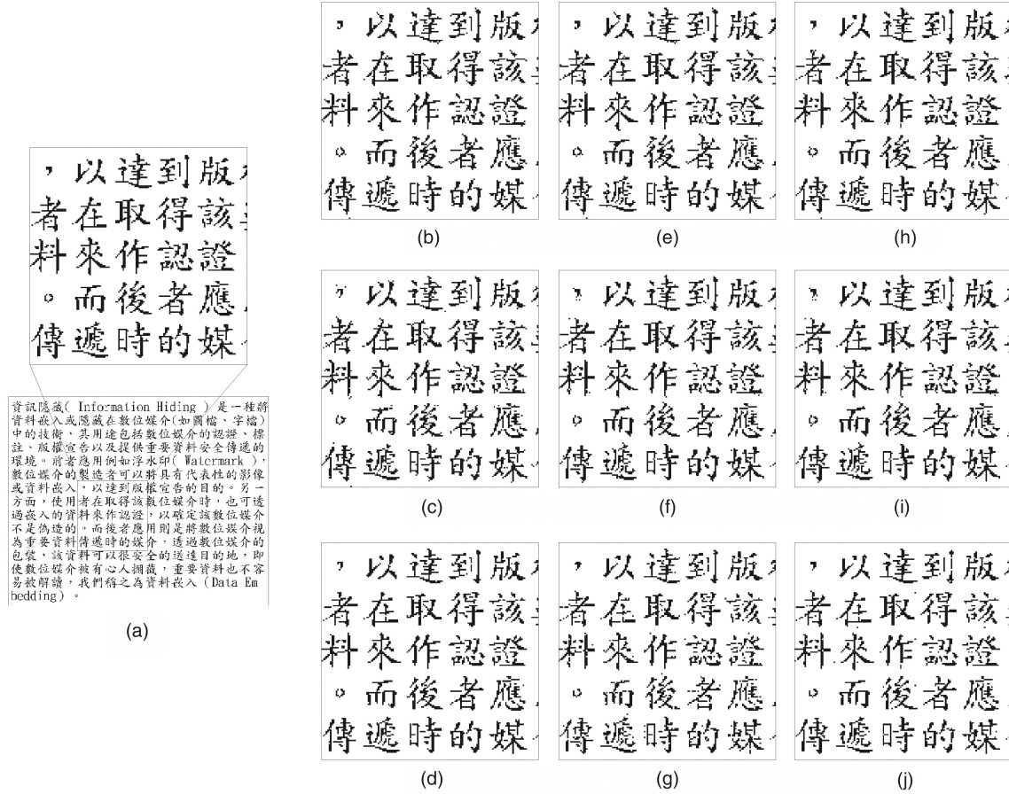
Fig. 4. Hiding effect on a Chinese document: (a) the original host image, (b) hiding 889 bytes by our new scheme with block size 12 \times 12 , (c) hiding 1,291 bytes by CPT scheme with block size 12 \times 12 , (d) hiding 190 bytes by WL scheme with block size 12 \times 12 , (e) hiding 933 bytes by our new scheme with block size 12 \times 12 , (f) hiding 933 bytes by CPT scheme with block size 16 \times 16 , (g) hiding 933 bytes by WL scheme with block size 4 \times 4 , (h) hiding 682 bytes by our new scheme with block size 16 \times 16 ,
