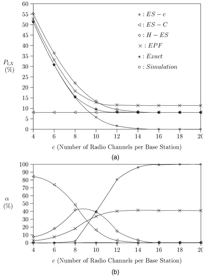
Fig. 6. Accuracy analysis of the analytic models ( $C = 42$ ,  $M = 6$ ,  $N = 100$ ,  $1/\mu = 3$  min, and  $\rho = 70m$  Erlang per ST). (a) Loss probability and (b) discrepancy of analytic models.
