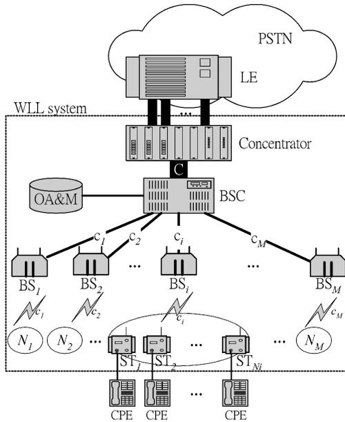
Fig. 1. A typical WLL architecture.
