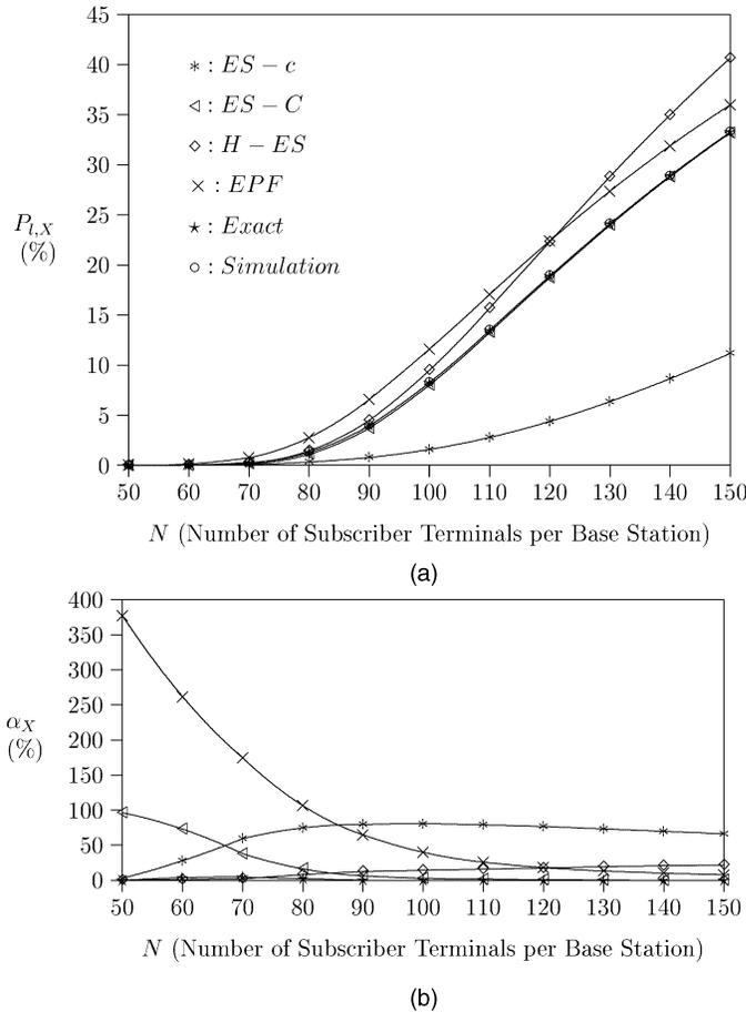
Fig. 5. Accuracy analysis of the analytic models ( $C = 42$ ,  $c = 12$ ,  $M = 6, 1/\mu = 3$  min, and  $\rho = 70m$  Erlang per ST). (a) Loss probability and (b) discrepancy of analytic models.
