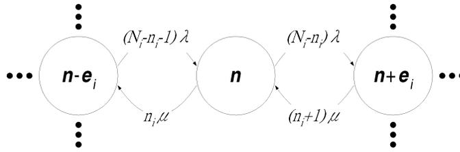
Fig. 2. Markov flow diagram for state  $\mathbf{n}$  ( $1 \leq i \leq M$ ).
