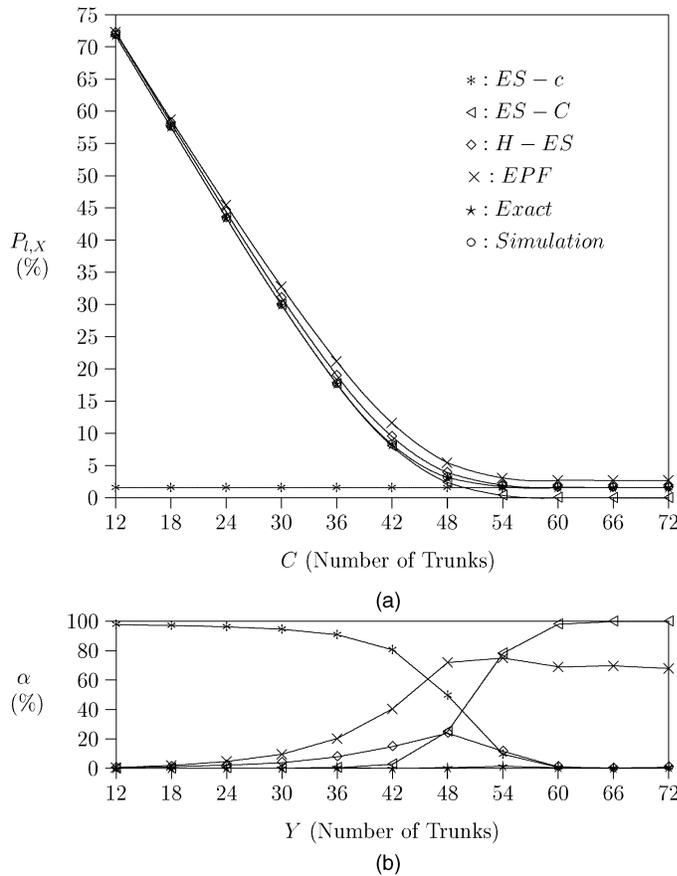
Fig. 7. Accuracy analysis of the analytic models ( $c = 12, M = 6, N = 100, 1/\mu = 3 \text{ min.}$ , and  $\rho = 70m$  Erlang per ST). (a) Loss probability and (b) discrepancy of analytic models.
