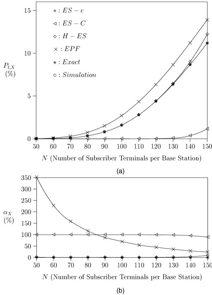
Fig. 4. Accuracy analysis of the analytic models ( $C = 72$ ,  $c = 12$ ,  $M = 6$ ,  $1/\mu = 3$  min., and  $\rho = 70m$  Erlang per ST). (a) Loss probability and (b) discrepancy of analytic models.
