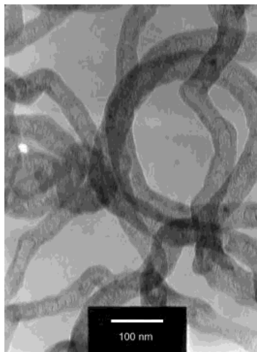
Fig. 3. Transmission electron microscope image of the multiwalled CNTs, produced by direct HFCVD.
