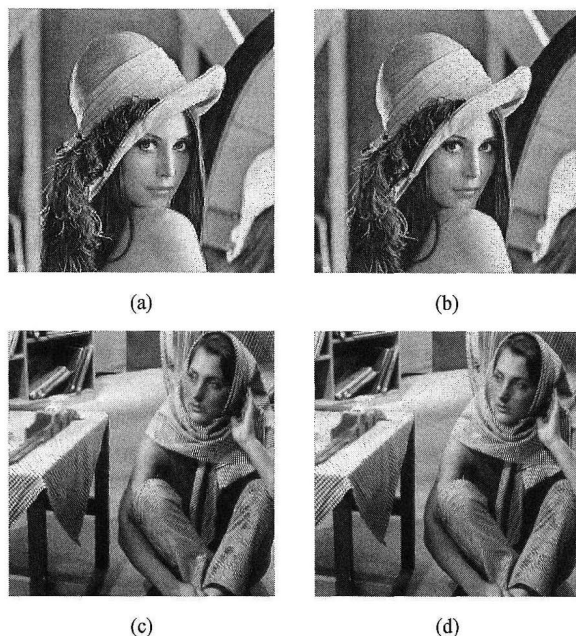
Fig. 7 Test on visibility of embedding of watermark (PSNR = 25.0 dB). (a) WTGM( S_2 ) watermarked Lena without HVS ( \alpha = 1.731 ). (b) WTGM( S_2 ) watermarked Lena with HVS ( \alpha = 9.741 ). (c) WTGM( S_2 ) watermarked Barbara without HVS ( \alpha = 0.872 ). (d) WTGM( S_2 ) watermarked Barbara with HVS ( \alpha = 3.374 ).
