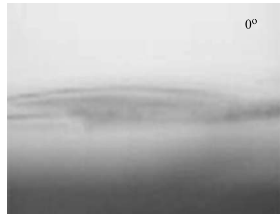
Fig. 8 A water drop on the surface of a thin film of TiO 2 (sample 2) with ATO nanochannel arrays showing zero contact angle without ultraviolet illumination
