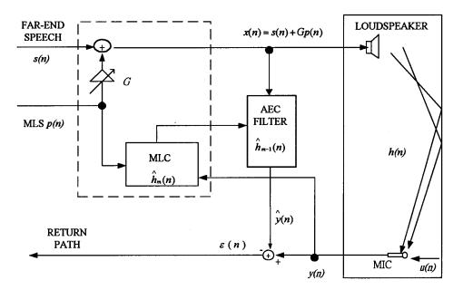
Fig. 2. AEC block digram with the masked MLC algorithm.
