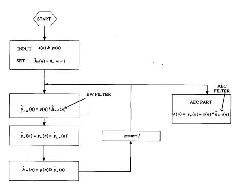
Fig. 3. Flowchart of the IMLC algorithm.
