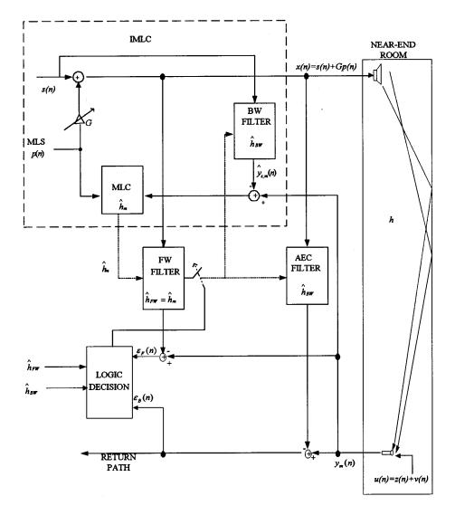
Fig. 8. Proposed IMLC AEC with DTD structure.
