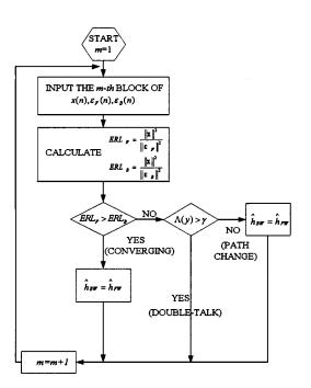
Fig. 7. Flowchart of DT detection based on the MAP rule.
