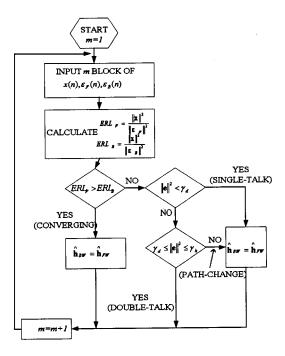
Fig. 10. Flowchart of proposed DT detection.
