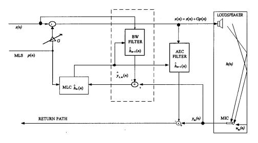
Fig. 4. IMLC AEC block diagram.
