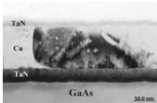
Fig. 4. Cross-sectional TEM micrograph of the TaN/Cu/TaN/GaAs sample after 550 °C annealing.
