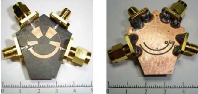
Fig. 7. Photos of the fabricated stepped-impedance rat race coupler with the broadside-coupled structure. (a) Top view. (b) Bottom view
