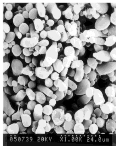
B PP/PBT/PP-MA(0.3)/Epoxy = 20/70/10/0.1 phr
