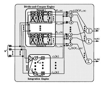
Fig. 2. The architecture of an MPN: (a) DCL engine, (b) IE, and (c) the output control logics [to the right of (a) and (b)].
