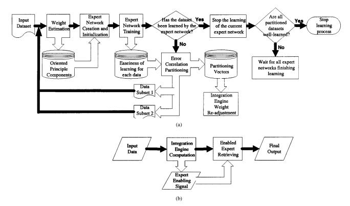
Fig. 1. DCL algorithm processes flow diagram. (a) Learning phase of the DCL modular perceptron network. (b) Retrieving phase of the DCL modular perceptron network.
