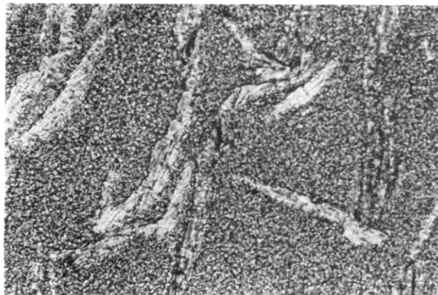
Figure 4. Optical polarizing micrographs displayed by IP: (A) S A texture obtained after cooling to 221 °C; (B) S C * texture obtained after cooling to 178 °C.
