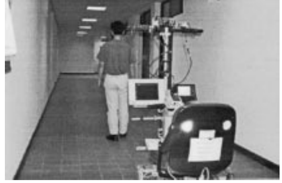
Fig. 9. The vehicle is guided automatically to follow a person who walks in front of the vehicle.
