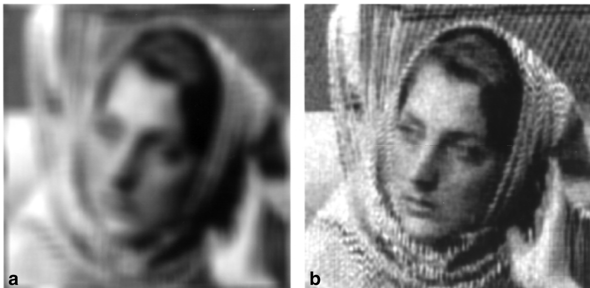
Fig. 1 (a) A blurred image of a woman. This image is blurred with a point spread function of 10 \times 10 pixels. (b) A deconvoluted image resulting from minimization of eq. (1).
