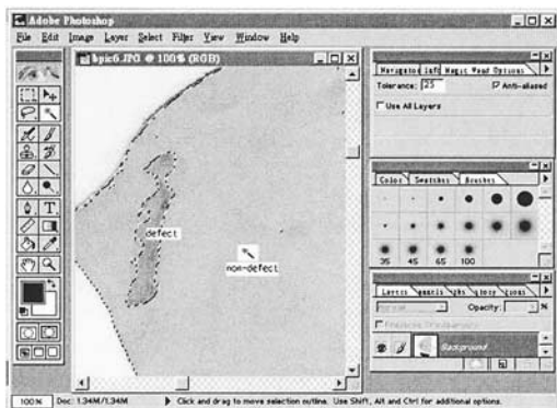
Fig. 4. Contamination image extraction by using a magic wand tool.
