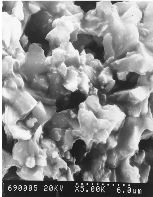
Figure 2. SEM micrograph of SiC p coated with Cu.
