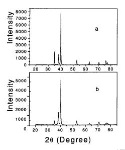
FIG.1 X-ray diffraction patterns of pure Ti (a) and Ti with 10 at. % A1 (b). The patterns show that no preferential orientation exists in these two samples.
