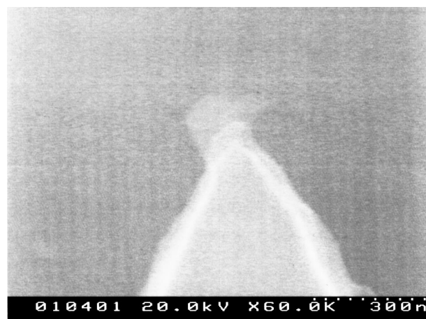
FIG. 3. High-resolution SEM micrograph indicating a tip radius below 55 nm.
