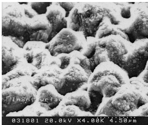
Fig. 7. SEM photo of the surface morphology of as-deposited In–Sn solder film.
