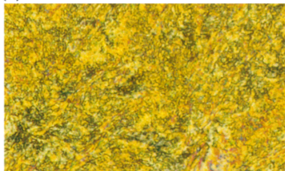
Figure 6. Polarized micrographs of (a) 30/70, (b) 50/50, and (c) 70/30 P64/PA6 blends annealed at 270 °C for 5 min.
