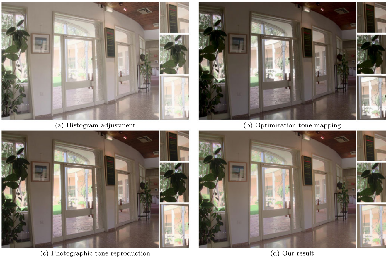
Fig. 7 DaniBelgium.hdr (radiance map courtesy of Karol Myszkowski). The result by histogram adjustment looks washed out. The leaf veins in our result are clearer than those in other results
