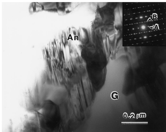
Fig. 6. Anorthite (marked "An") in the sample after exposure at 1200°C for 500 h; SADP was identified as a mixture of C \bar{1} anorthite and P \bar{1} anorthite, with the twin plane parallel to (010) (A = (020) and B = (022)); region marked "G" is a glassy phase.
