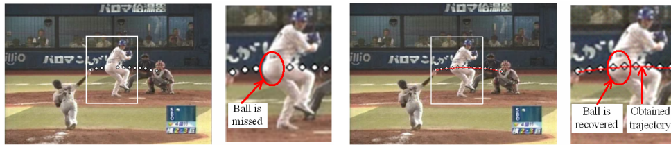
(a) Ball detection. Two ball positions are missed when passing over the white uniform. (b) Ball tracking. Positions of missed balls can be recovered.
