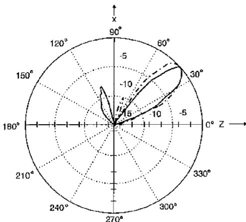
**Fig. 9**  $H$ -plane ( $x$ - $z$ -plane) radiation patterns of  $4 \times 1$  active microstrip leaky-wave antenna array, for  $f = 8.95\text{GHz}$
