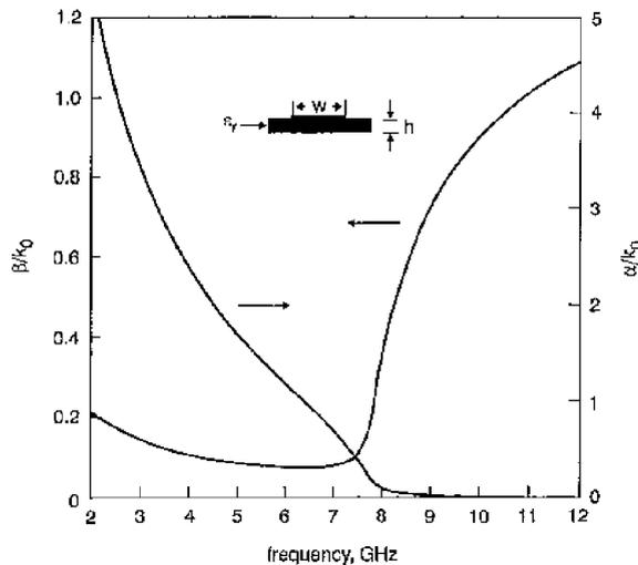
**Fig. 7** Normalised propagation constant of first higher-order mode for particular microstrip leaky-wave antenna
