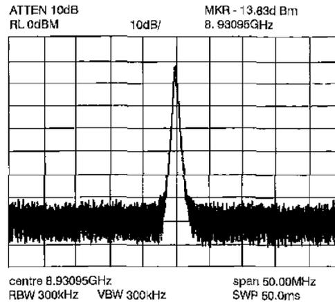
**Fig. 5** Spectrum of  $4 \times 1$  active antenna array measured at 8.93GHz
