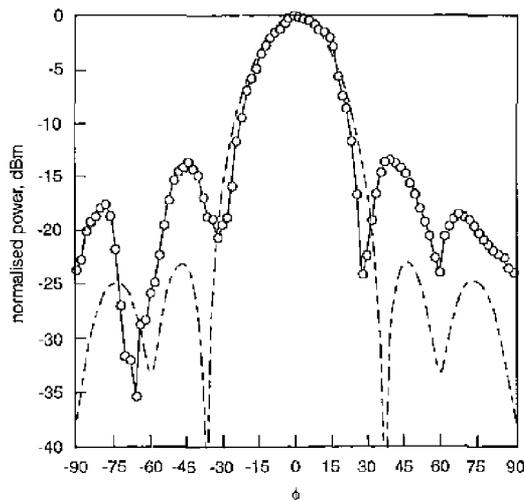
**Fig. 12** Measured and theoretical patterns for  $\Delta\phi = 0^\circ, f = 8.731\text{GHz}$
