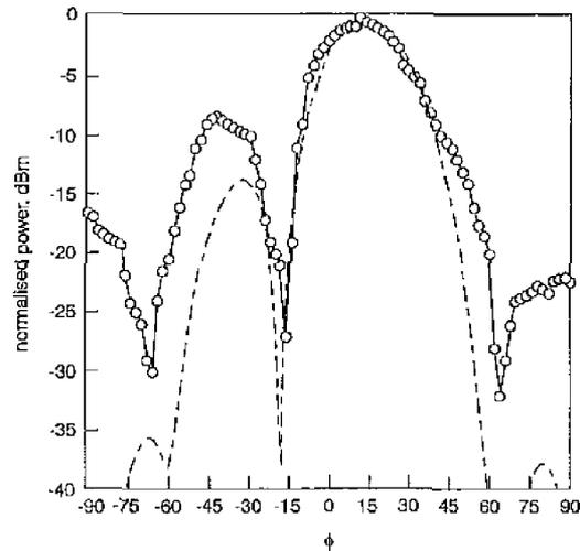
**Fig. 13** Measured and theoretical patterns for  $\Delta\phi = 40^\circ, f = 8.723\text{GHz}$
