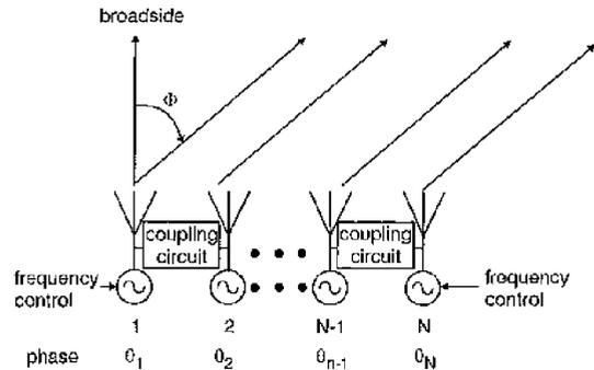
**Fig. 10** Block diagram of  $N$  coupled-VCO phased-array system for beam scanning
