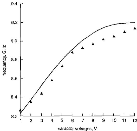
**Fig. 4** Active varactor-tunable leaky-wave antenna array results: simulated and measured varactor tuning frequency against voltage
