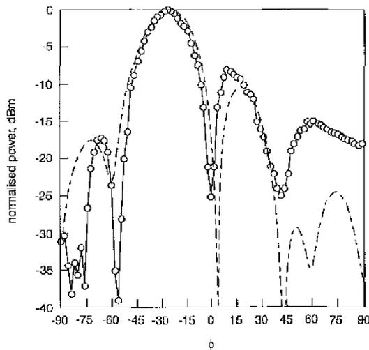
**Fig. 11** Measured and theoretical patterns for  $\Delta\phi = 80^\circ, f = 8.739\text{GHz}$
