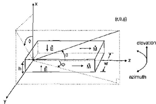
**Fig. 6** Geometry and co-ordinate system for microstrip leaky-wave antenna
