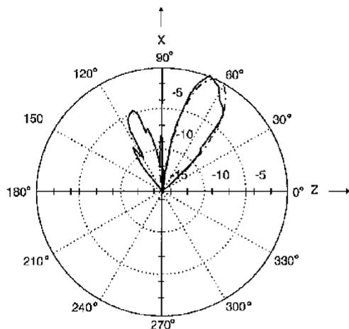
**Fig. 8**  $H$ -plane ( $x$ - $z$ -plane) radiation patterns of  $4 \times 1$  active microstrip leaky-wave antenna array, for  $f = 8.24\text{GHz}$
