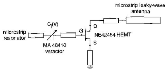
**Fig. 3** Schematic diagram for varactor-tuned VCO
