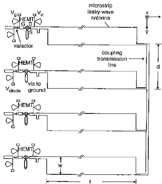
**Fig. 1** Configuration of  $4 \times 1$  active microstrip leaky-wave antenna array  $w = 12\text{mm}$ ;  $l = 100\text{mm}$ ;  $d = \lambda_x$  at 8.8GHz
