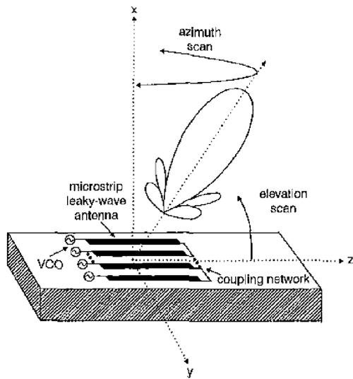
**Fig. 2** Schematic diagram of two-dimensional scanning using linear active phased array of leaky-wave line sources
