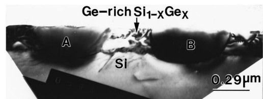
FIG. 2. XTEM image of the \text{Ni}/\text{Si}_{0.76}\text{Ge}_{0.24} sample annealed at 500 °C showing the agglomeration structures. The grains denoted as “A” and “B” are of \text{Ni}(\text{Si}_{1-x}\text{Ge}_x) .
