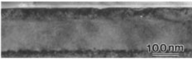
Fig. 5. Cross-sectional view of specimen 221 annealed at 600°C for 1 h.
