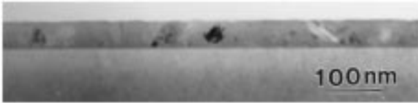
Fig. 1. Cross-sectional of specimen containing 60 nm LPCVD film without ion implantation annealed at annealed at 600°C for 2 h.
