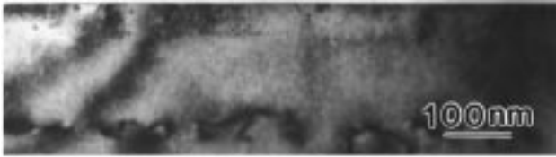
Fig. 10. The BF cross-sectional view micrographs of specimen 23 annealed at 1000°C for 10 min.
