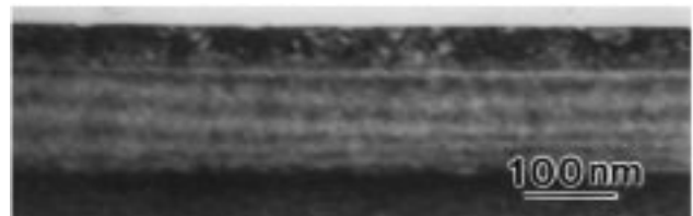
Fig. 7. Cross-sectional view of specimen 22 subjected to ICPO modification and annealed at 600°C for 4 h.
