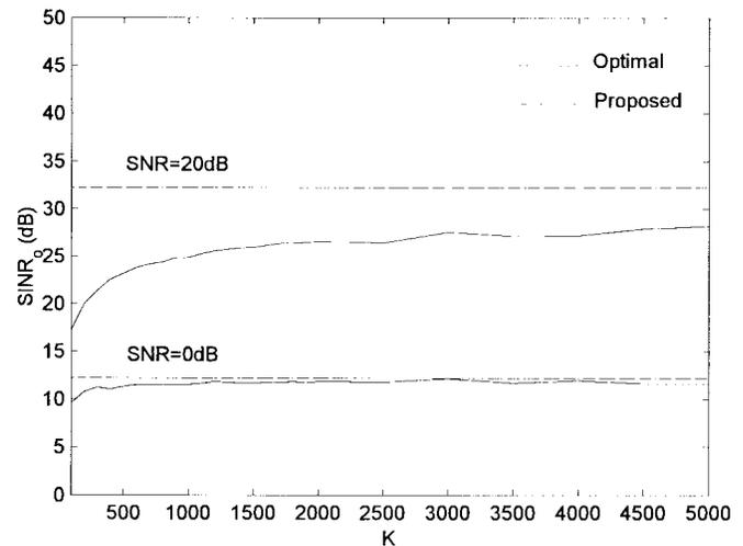
Fig. 8. Convergence behavior of proposed combiner with SNR = 0 and 20 dB.
