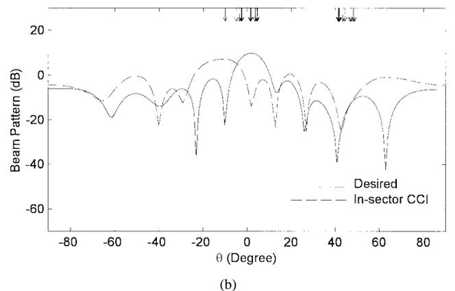
Fig. 7. Performance of proposed combiner in the presence of in-sector CCI. (a) Output SINR versus  $\theta_1$ . (b) Pattern obtained with  $\theta_1 = -10^\circ$ .
