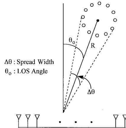
Fig. 2. Geometry of local scattering model.
