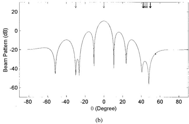
Fig. 6. Performance of proposed combiner as a function of angle spread. (a) Output SINR versus  $\Delta\theta$ . (b) Pattern obtained with  $\Delta\theta = 0^\circ$ .
