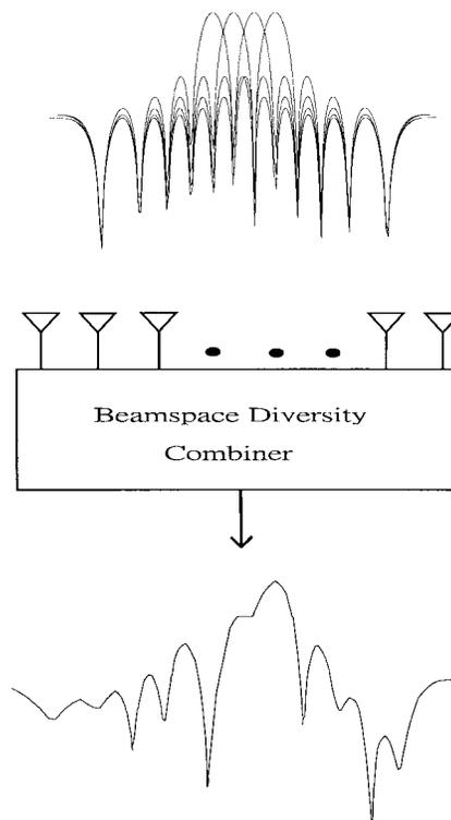
Fig. 1. Illustration of proposed diversity combining scheme.
