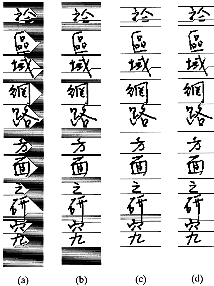
Fig. 6. Results of redundant segmentation path removal: (a) image after detecting all possible segmentation paths; (b) image after removing overlapping paths; (c) image after eliminating redundant path in gaps; (d) image after discarding near paths.
