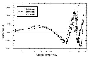
Fig. 2. Relative noise power fluctuations versus input optical power for three wavelengths.
