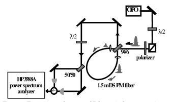
Fig. 1. Experimental setup: OPO, optical parametric oscillator;  $\lambda/2$ 's, half-wave plates; DS PM, dispersion-shifted polarization-maintaining.
