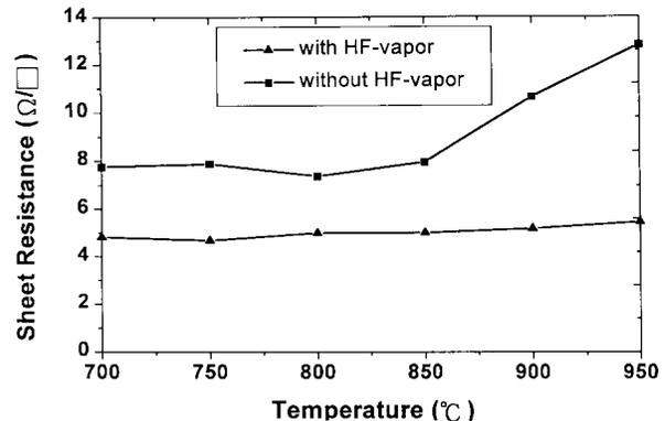
Fig. 1. Sheet resistance of CoSi<sub>2</sub> on p<sup>+</sup>n junction with different surface treatment.
