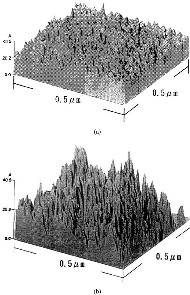
Fig. 3. STM images of (100) Si surface treated (a) with and (b) without HF-vapor before metal deposition.
