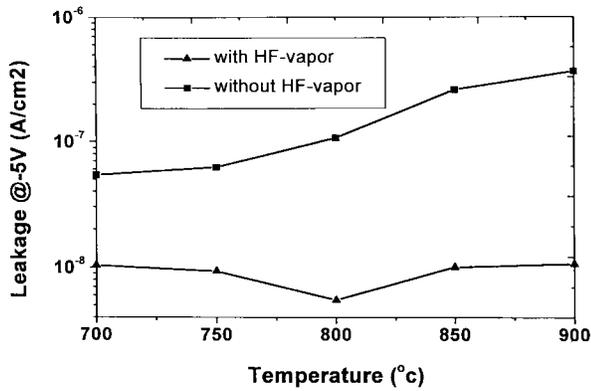
Fig. 2. Leakage current of p<sup>+</sup>n junction with different surface treatment.
