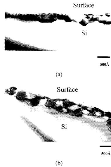
Fig. 4. Cross-sectional TEM images of CoSi<sub>2</sub> film treated (a) with and (b) without the HF-vapor before metal deposition.
