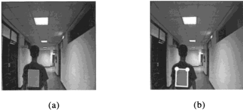
Figure 6. The experimental result of feature point detection. (a) is a captured image with the segmented rectangular shape. (b) Detected feature points.
