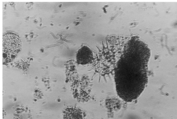
Fig. 2. Photomicrograph ( 250\times ) of the 5th-day sludge particles showing the bio-flocculation with Pediastrum .
