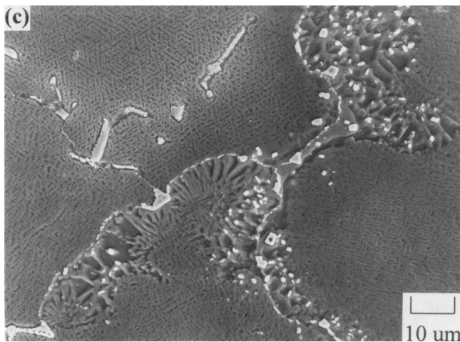
Fig. 1—Microstructures of a Mg-free MAR-M247 superalloy after heat treatment: (a) morphology of \gamma' phase, (b) morphology of \gamma - \gamma' eutectic structure, and (c) MC scrip-like carbides within the grain interior and M_{23}C_6 carbides at the grain boundary.
