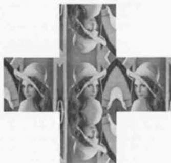
Fig. 2. Circular extension and symmetric extension. (a) circular extension in a sequence (b) symmetric extension in a sequence (c) circular extension of image edges (d) symmetric extension of image edges.
