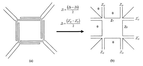
Figure 3 (a) Physical diagram of dc block branch-line coupler. (b) Single-line equivalent circuit
