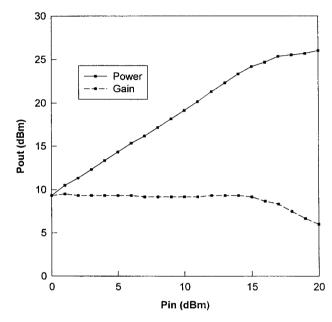
**Figure 6** Measured power performance and gain of balanced amplifier at 10 GHz
