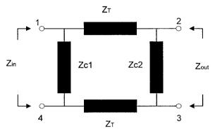
Figure 1 Impedance-transforming branch-line coupler
