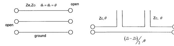
Figure 2 Coupled line equivalent to single line [3]
