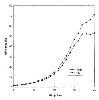
Figure 7 Efficiency performance of the balanced amplifier
