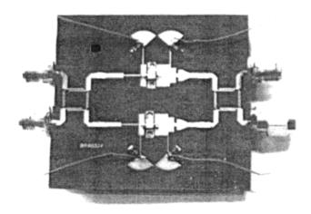
**Figure 5** Photograph of the fabricated balanced amplifier
