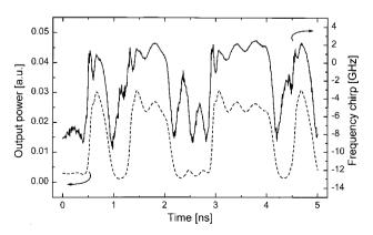
Figure 3 Time traces of the modulated laser output power and the measured frequency chirp for a DFB laser operating at 1.55  $\mu m$
