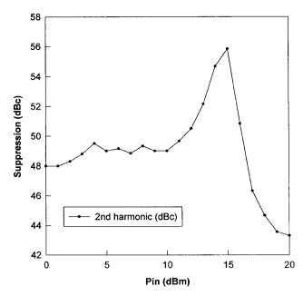
Figure 8 Output second harmonic versus input power of the balanced amplifier
