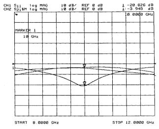
Figure 4 Measured small-signal performance of the coupler
