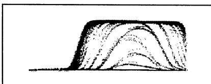
Fig. 14. The beam map of an uncentered beam scan with a vertically imbalanced scan amplitude.
