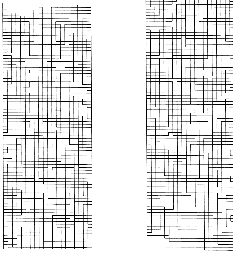
Fig. 10. Routing result for Deutsch's difficult example.
