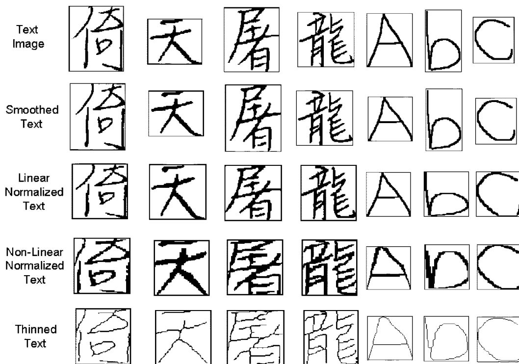
Fig. 4. Image preprocessing on handwritten characters: (from top) original text image, smoothed text, linear normalized text, nonlinear normalized text and thinned text.
