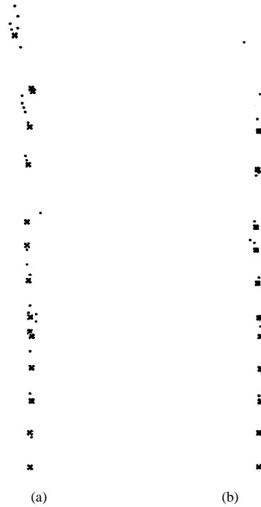
Fig. 11. An example of learned global models: (a) initial learned model and (b) refined model after five iterations of incremental-learning-by-navigation. The crosses represent real vertical lines and the spots are noise. Note the removal of some noise points.
