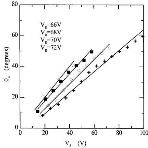
Fig. 7. The plots of the computed values of  $\theta_a$  versus  $V_a$  which are computed from the data of Fig. 6 and the measured gate currents based on (8) for several gate voltages. Four plotted curves are roughly linear and their extrapolated points intersect at the horizontal axis at  $V_a \cong 0, 4,$  and  $6$  V for  $V_g \leq 68$  V,  $= 70$  V and  $= 72$  V, respectively.
