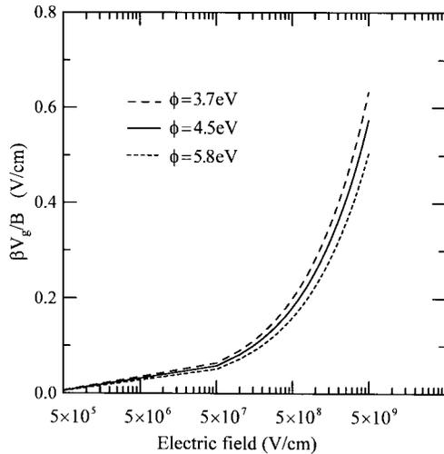
Fig. 4. The value of the term,  $\beta V_g/B$ , computed for several work functions. The value of this term is smaller than one even the electrical field is up to  $5 \times 10^9$  V/cm.
