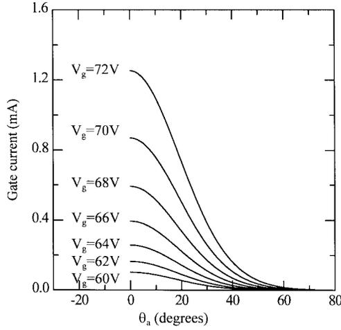
Fig. 6. The computed gate current as a function of the emission angle  $\theta_a$  from (8) for different gate voltages.
