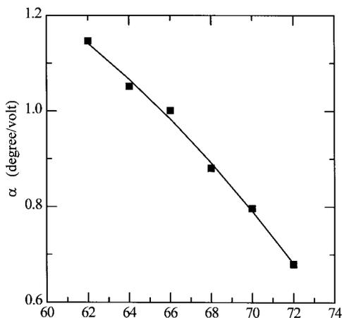
Fig. 11. The extracted  $\alpha$  as a function of  $V_g$  for the experimental device of [11]. The square dots are the extracted data and the solid line is the fitted curve for (10).
