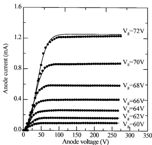
Fig. 13. The reconstructed current data (the solid curves) computed from the extracted values of the model parameters and the original measured data (the dotted curves). Two sets of characteristics match very well.
