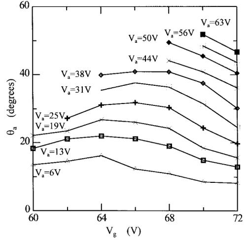
Fig. 8. The plots of  $\theta_a$  versus  $V_g$  computed by using (8) from Fig. 6 and the measured gate currents but with  $V_a$  as the varying parameters.  $\theta_a$  increases first then decreases with respect to  $V_g$  for all  $V_a$ .
