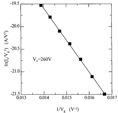
Fig. 10. The  $\ln(I_c/V_g^3)$  versus  $1/V_g$  plot of the cathode current of the experimental device operating at  $V_a = 260 \text{ V}$ . It is a closely approximated straight line as  $\ln(I_c/V_g^3) = \ln(6.27 \times 10^{-5}) - (708/V_g)$ .
