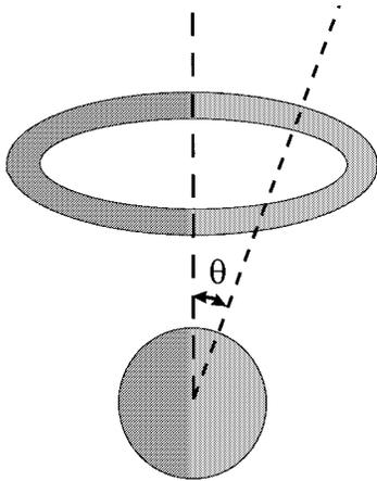
Fig. 1. The ‘‘Saturn’’ model, given by Jensen *et al.*, in which the tip is a floating sphere suspended near a ring of charge along the symmetry axis.
