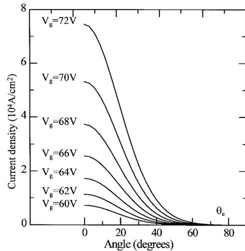
Fig. 2. The angular current density distribution calculated from (1)–(3) for several gate voltages.  $\theta_e$  is the critical emission angle beyond which the emission becomes negligible. The larger the  $V_g$ , the larger the  $\theta_e$ .
