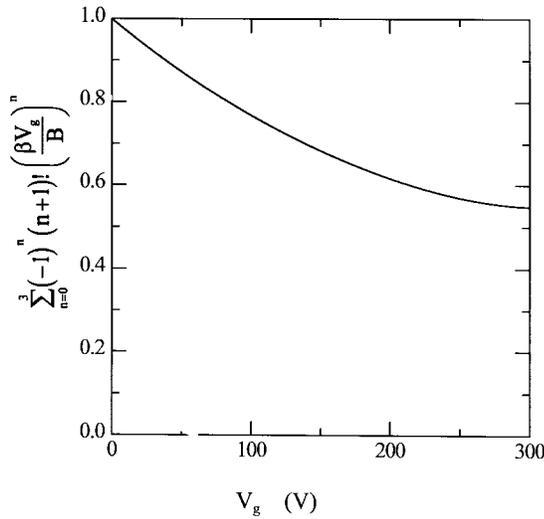
Fig. 9. The computed summation of the first four terms of the summation part,  $\sum_{n=0}^3 (-1)^n (n+1)! (\beta V_g/B)^n$ , of the parameter  $A'$  as a function of  $V_g$  for  $\beta = 9.25 \times 10^5 \text{ cm}^{-1}$  and  $\phi = 4.5 \text{ eV}$ . It is a slowly varying function of  $V_g$  for the whole 0–300 V gate voltage region.
