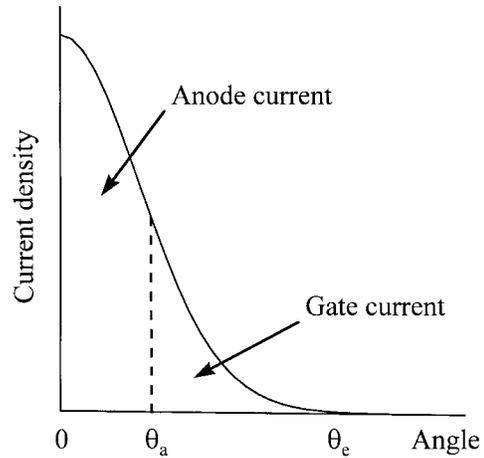
Fig. 5. The anode current component and the gate current component obtained from the current density distribution along the cathode surface respectively.  $\theta_a$  is the angle beyond which the cathode emitted charges are collected by the gate to be the gate current. The anode collects emitted currents emitted from the cathode for the angles from  $\theta = 0$  to  $\theta_a$ .
