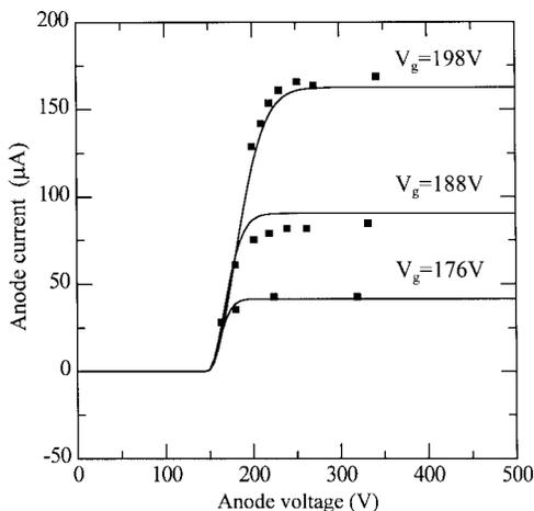
Fig. 14. The  $I$ - $V$  characteristics of an FET triode with 100 emitter tips. The square curves are the measured data which were obtained from the Holland's paper [28]. The solid lines are the reconstructed curves from the model.
