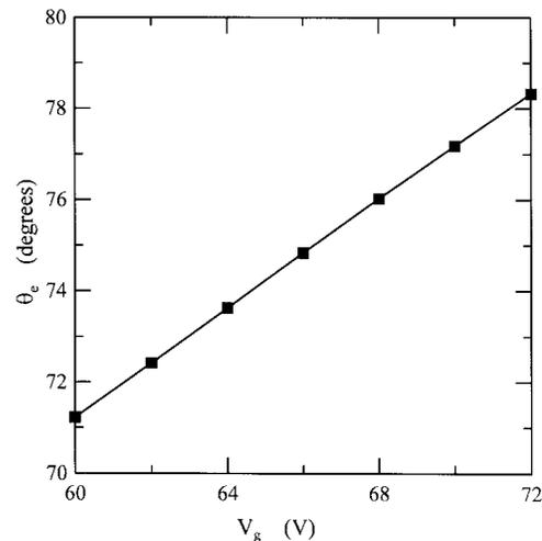
Fig. 3. The computed value of  $\theta_e$  in terms of  $V_g$  from (1)–(3). The  $\theta_e$  is defined as  $J(\theta = \theta_e) = 0.1\%J(\theta = 0)$ . The value of  $\theta_e$  is almost linearly proportional to  $V_g$ .
