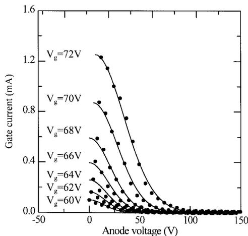
Fig. 12. The reconstructed gate current (the solid curves) and the measured data (the dotted curves) versus  $V_a$ .
