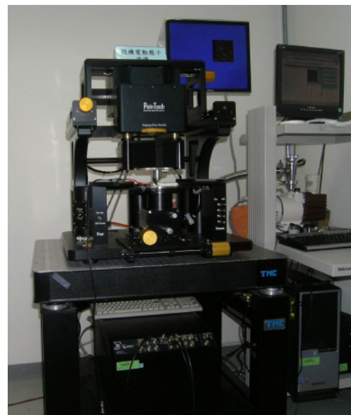
Fig. 7. (Color online) MEMS motion analyzer.
