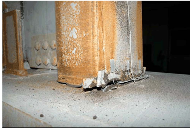
(a) Specimen IFS1 (Top Flange)
